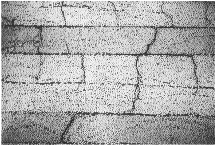
Figure 11 Extensive intra- and inter-laminar cracking corresponding to point F of Fig. 9.
